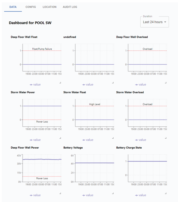
Plexus Console web application displaying real-time & 24hr historical data for RSL Tobruk
